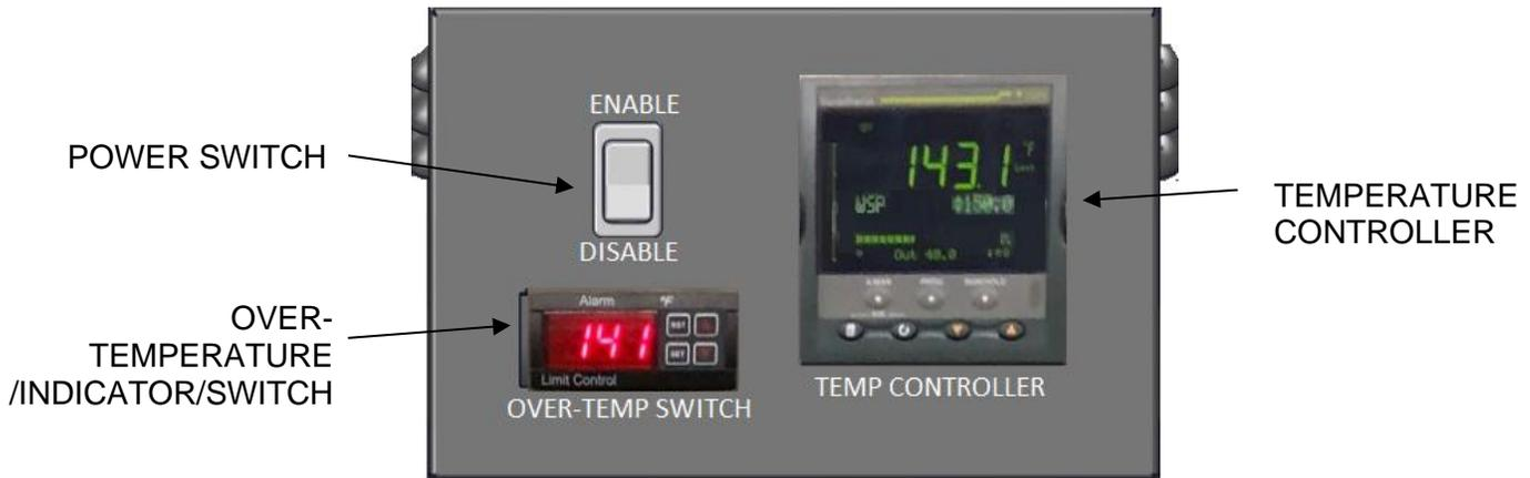
**Figure 4-5: Control Box – Front View**
