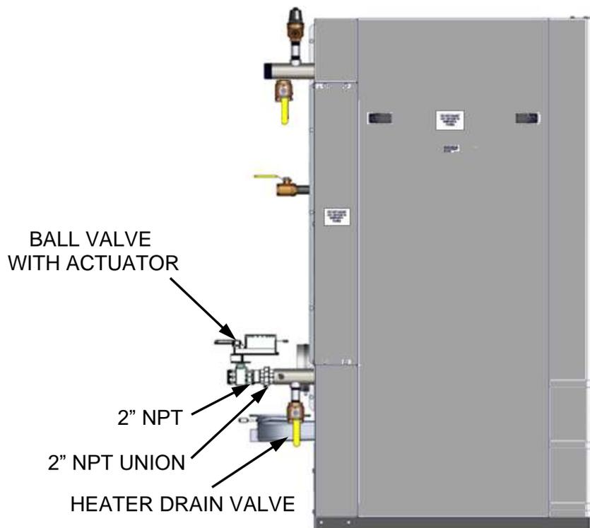
**Figure 2.5.1: Innovation Water Heater Equipped with Sequencing Valve**
