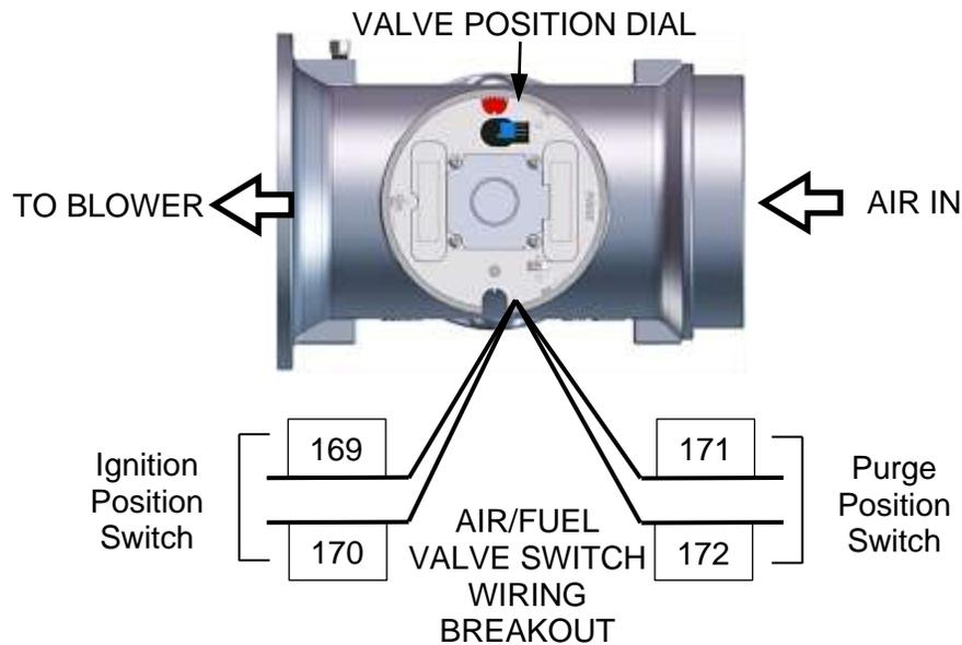
**Figure 5.11-2: Air/Fuel Valve Purge and Ignition Switch Locations**
