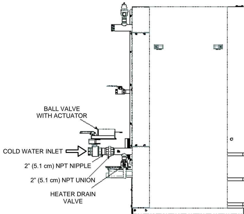
**Figure 8.7.2: Innovation Water Heater Equipped with Sequencing Valve**
