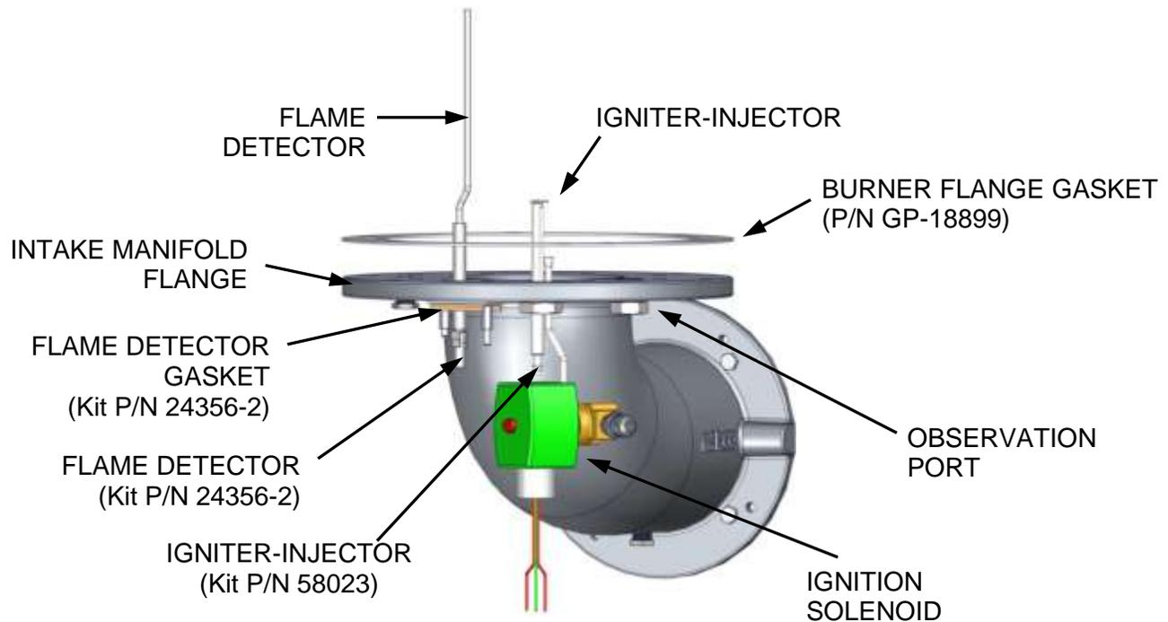
**Figure 6.3-1: Intake Manifold with Igniter-Injector & Flame Detector**
