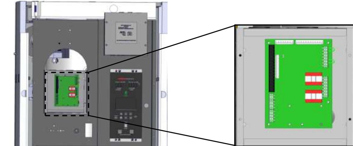
**Figure 2.12-1: Input/Output (I/O) Box Location – Partial Front View**
