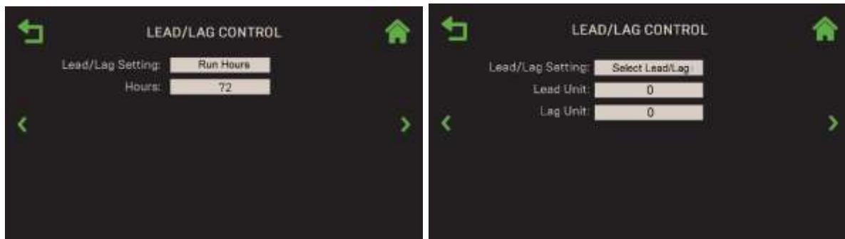
**Figure 8.6-7: Operating Controls: Lead/Lag Control Screen**
