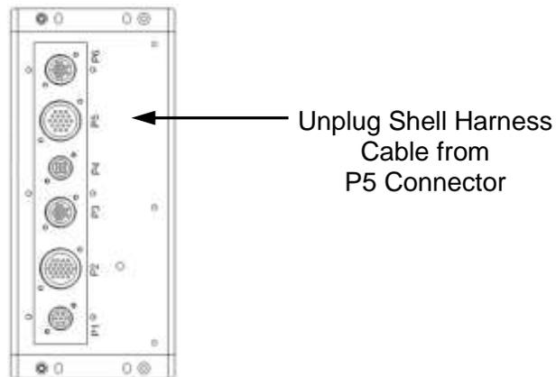
**Figure 6.11.1-1: Removing Shell Harness Cable from P5 Connector on Rear Panel**
