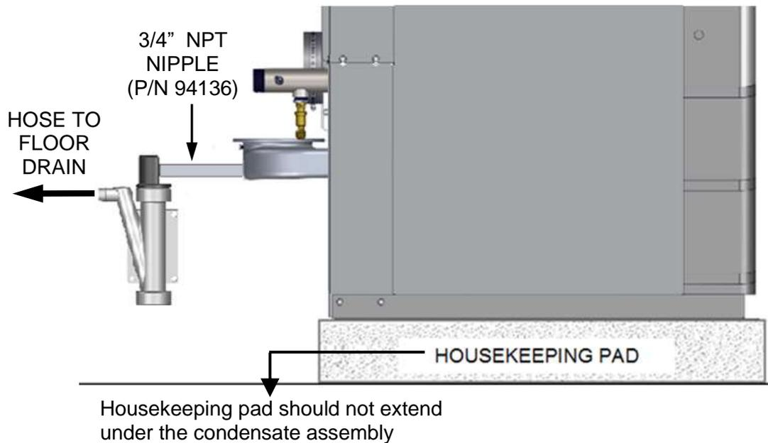
**Figure 2.9-2: Sample Condensate Trap Installation – Left Side View**
