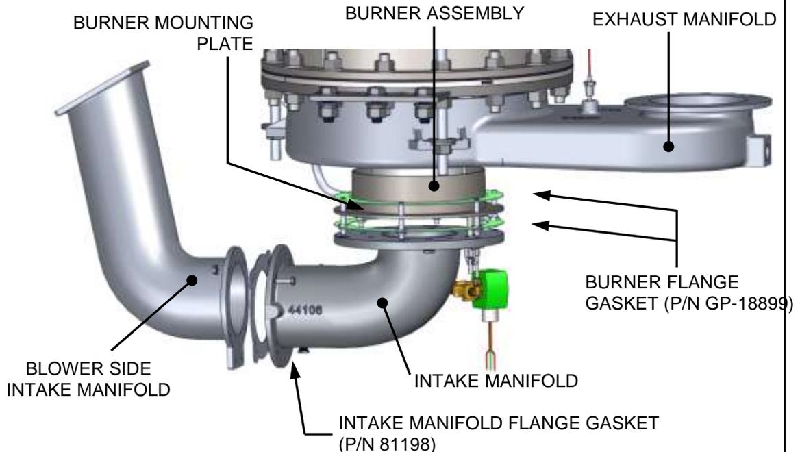
BURNER, INTAKE AND EXHAUST MANIFOLDS
