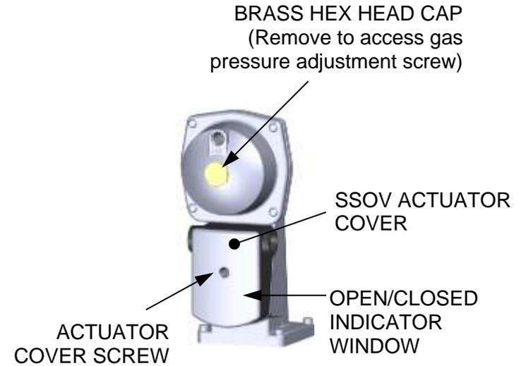
**Figure 7.2-3: SSOV Actuator with Gas Pressure Adjustment**
