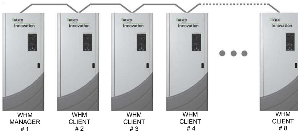
**Figure 8.7.3: Typical Daisy-Chain Modbus/RS485 Network**
