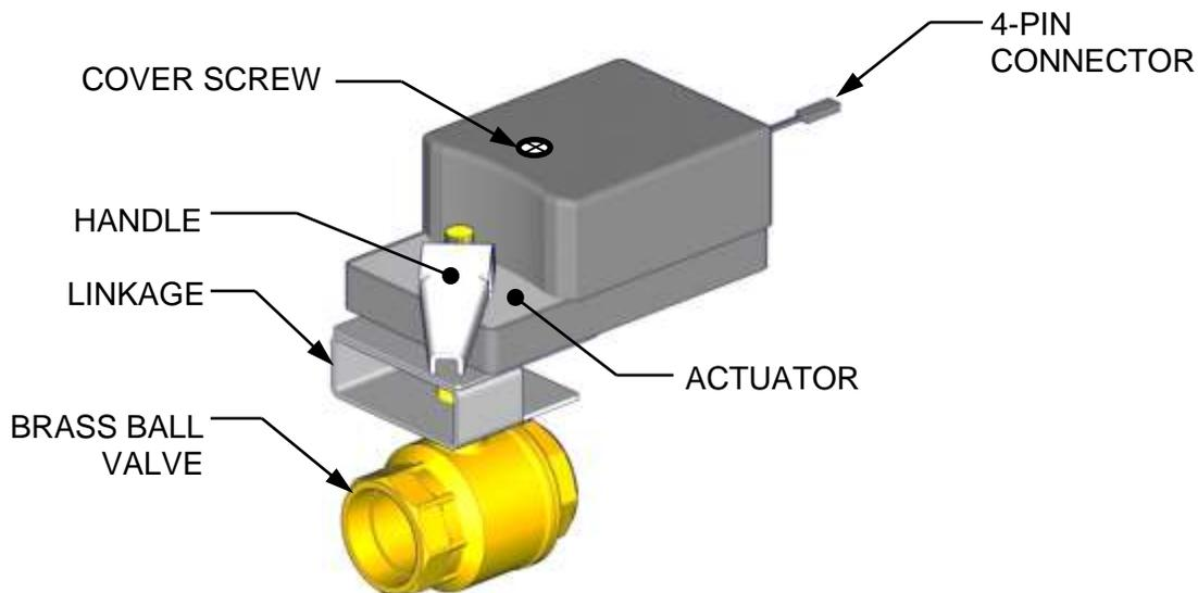
**Figure 8-10.1-1: Actuator-Controlled Sequencing Valve (P/N 92123)**
