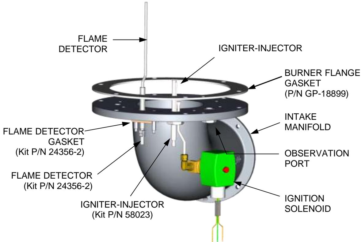
**Figure 7.2-2: Intake Manifold**
