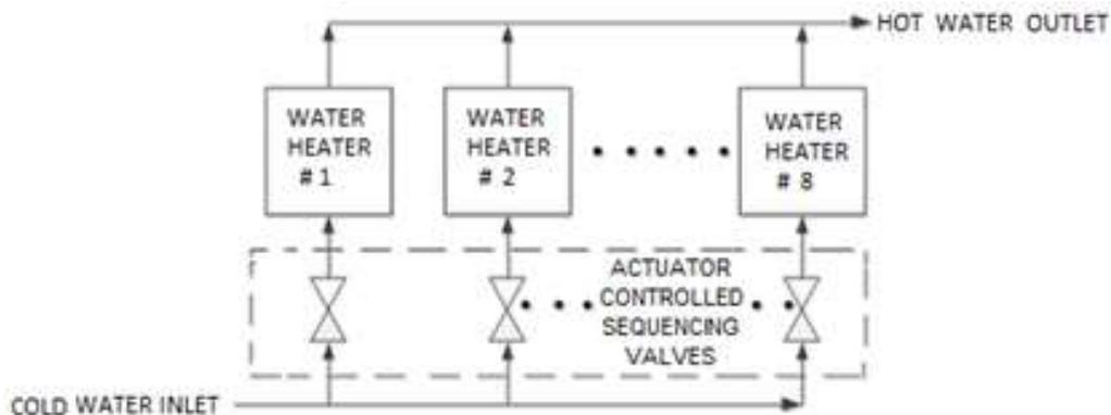
**Figure 8.1: Simplified Block Diagram - Water Heater Management (WHM)**
