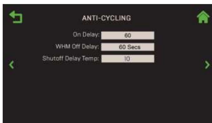
Figure 8.6-5: Operating Controls: Anti-Cycling Control Screen
