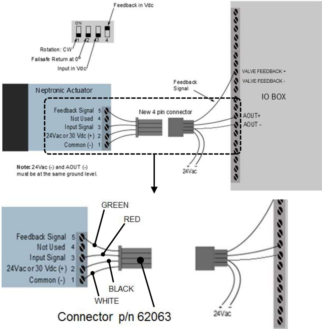
**Figure 8.10.2: Sequencing Valve Wiring**
