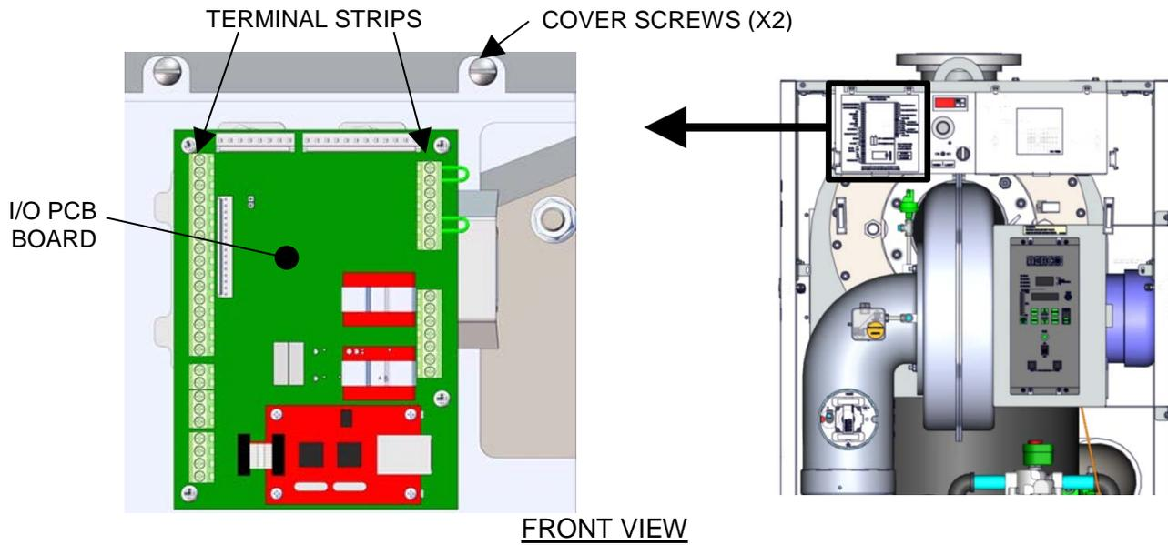
**Figure 2-12. Input/Output (I/O) Box Location**
