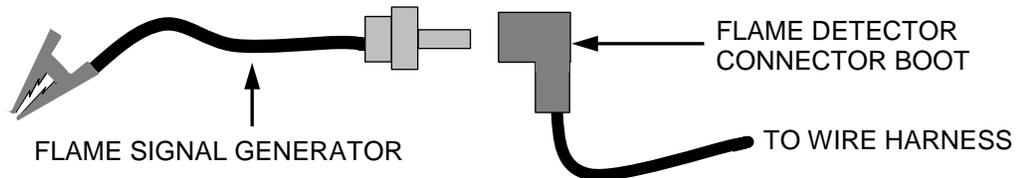
**Figure 6.6: Connecting the Flame Signal Generator**
