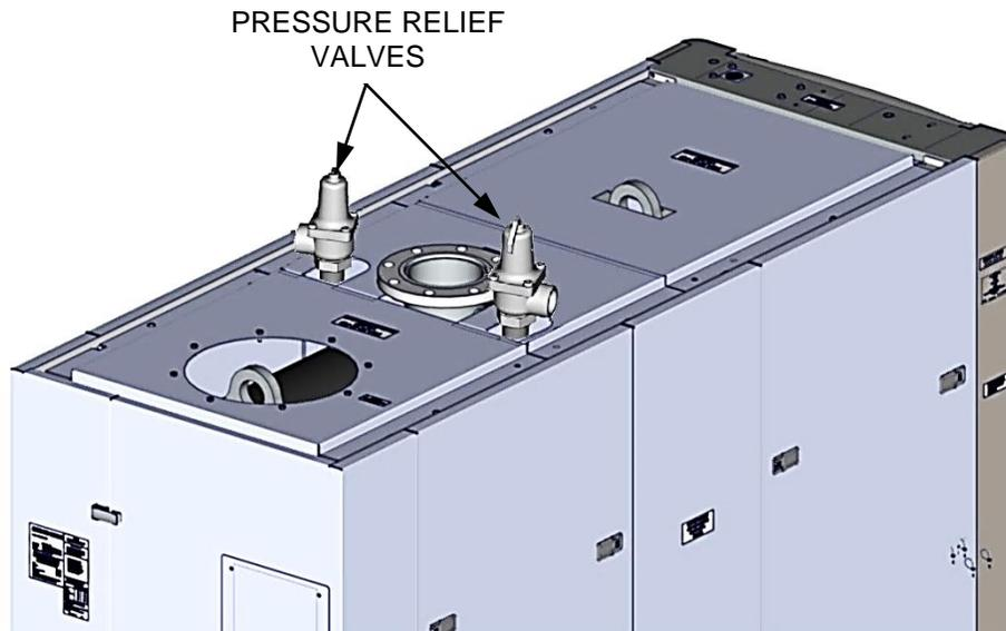
**Figure 2-5A: Pressure Relief Valve Installation Locations**
