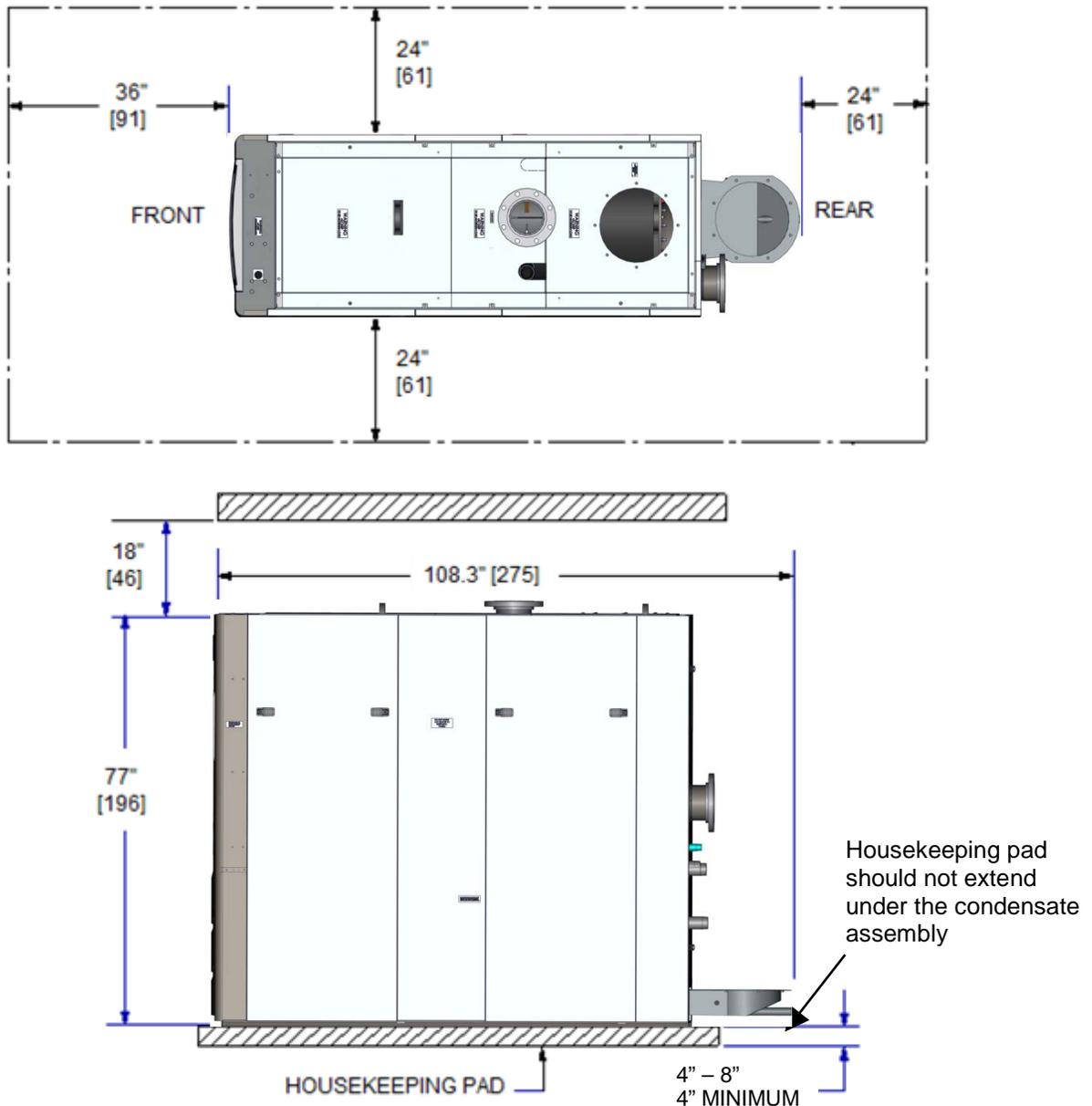
**Figure 2-2a. Benchmark Boiler Model 6000 Clearances**
