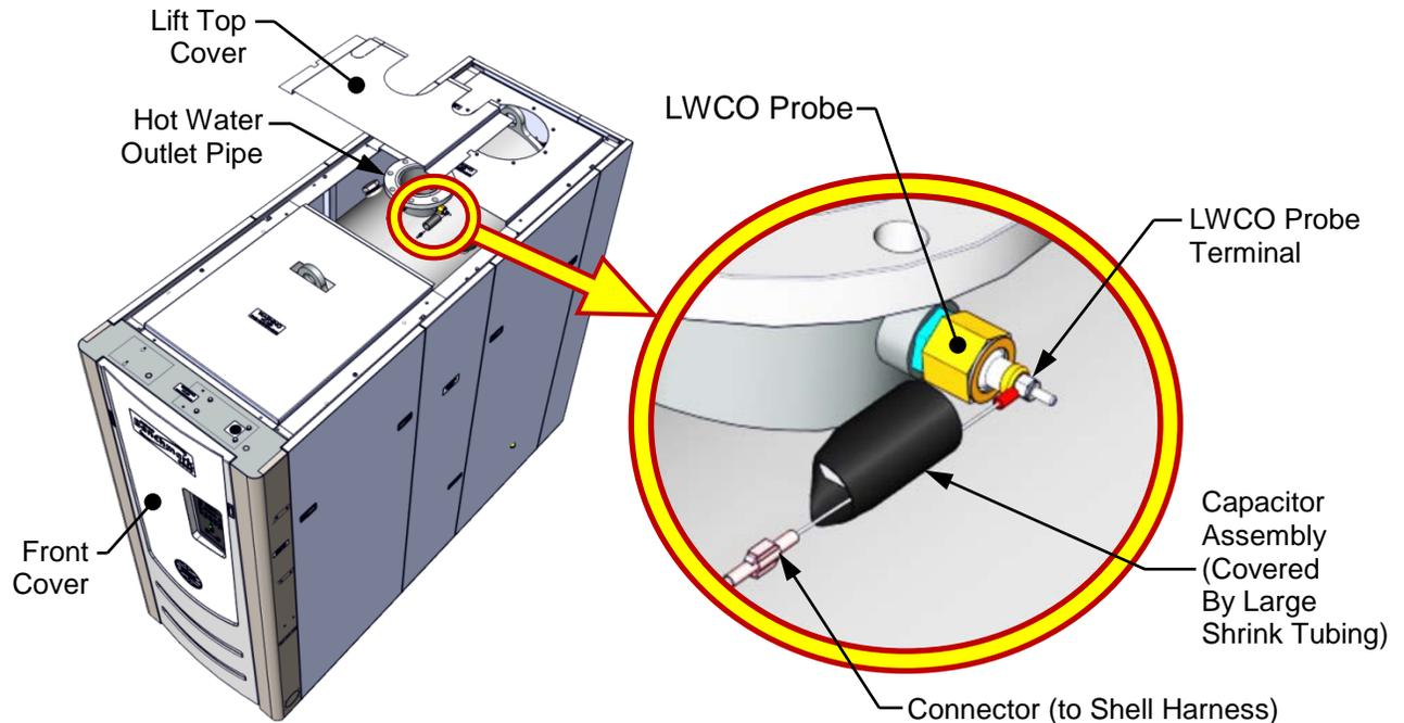
**Figure 7-12: LWCO Probe Location for BMK6000**
