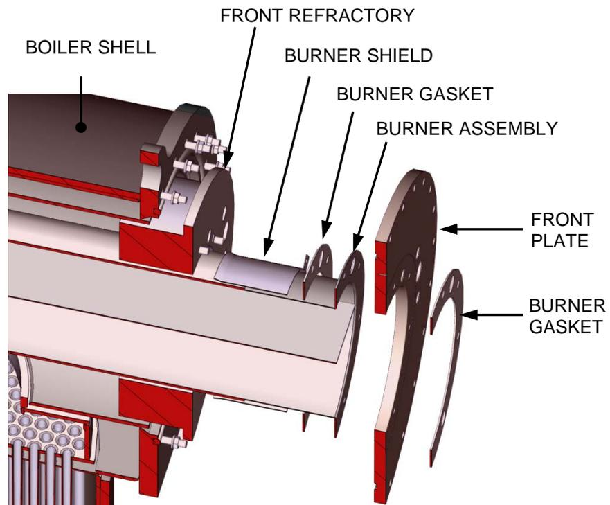
**Figure 7-9b: Front Plate Assembly – Cut-Away View**
