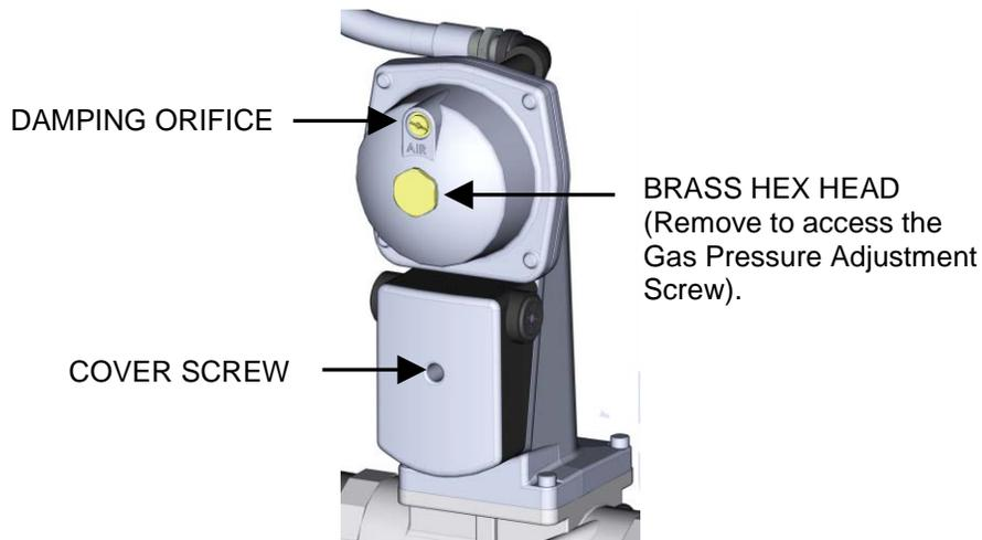
Figure 8-3: SSOV Actuator With Gas Pressure Adjustment (SKP25)
