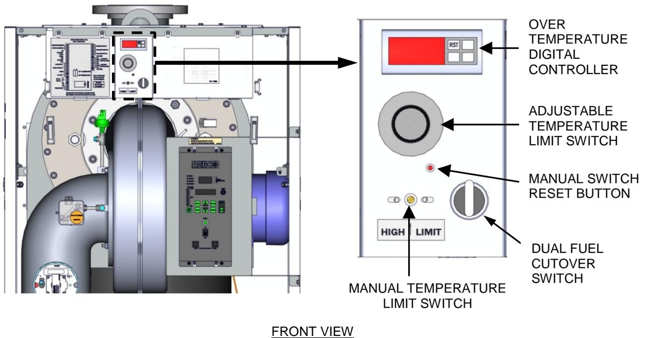
**Figure 6-3: Temperature Limit Switch Setting**
