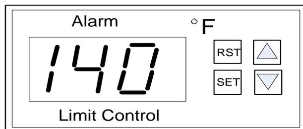
**Figure 4-6: Digital Over-Temperature Alarm Switch Front Panel**
