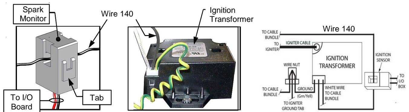
**Figure 7-15: Spark Detector Sensor (AC Current Transducer) P/N 61034**
