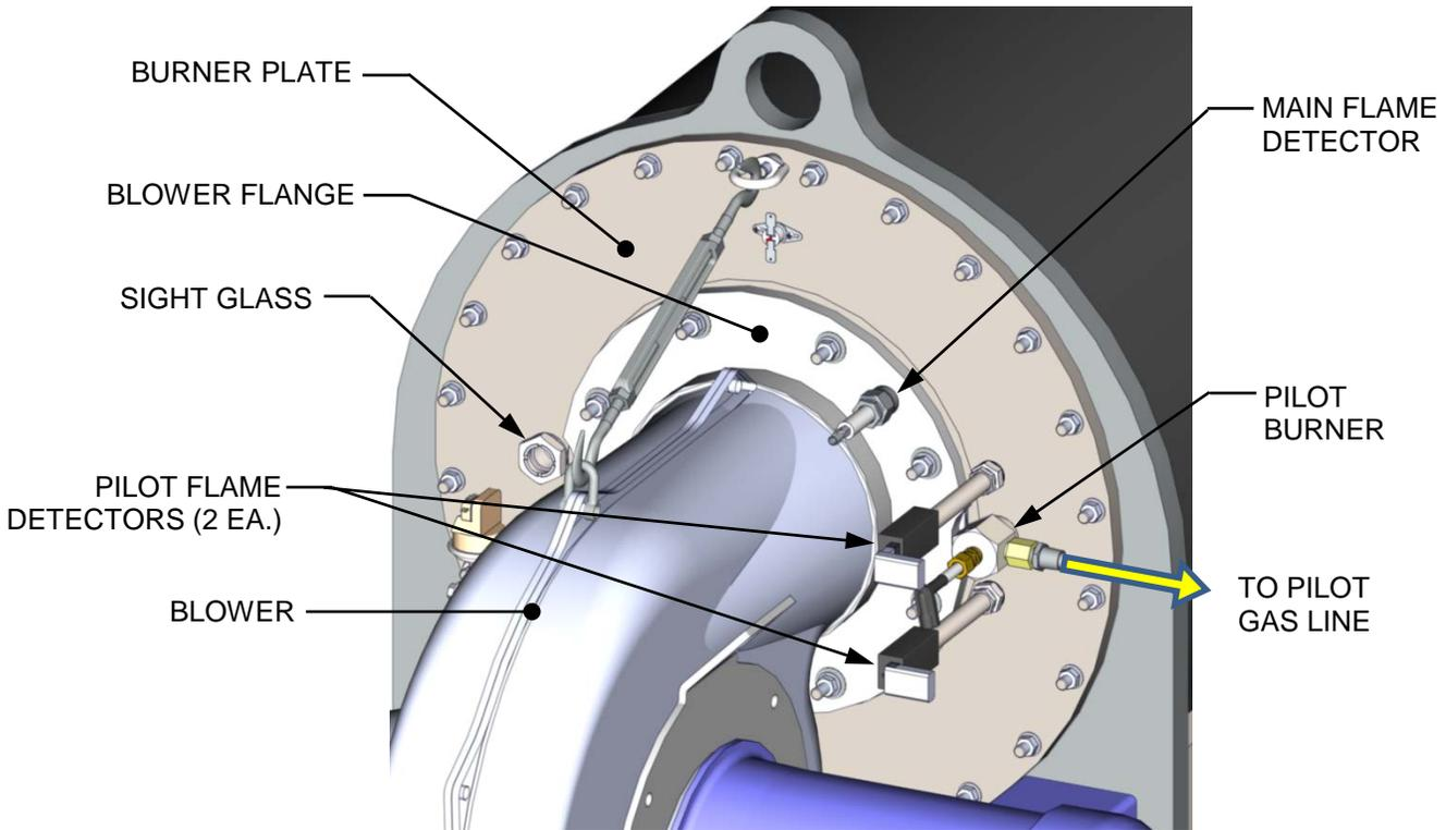
Figure 8-2: Pilot Burner & Flame Detector Locations
