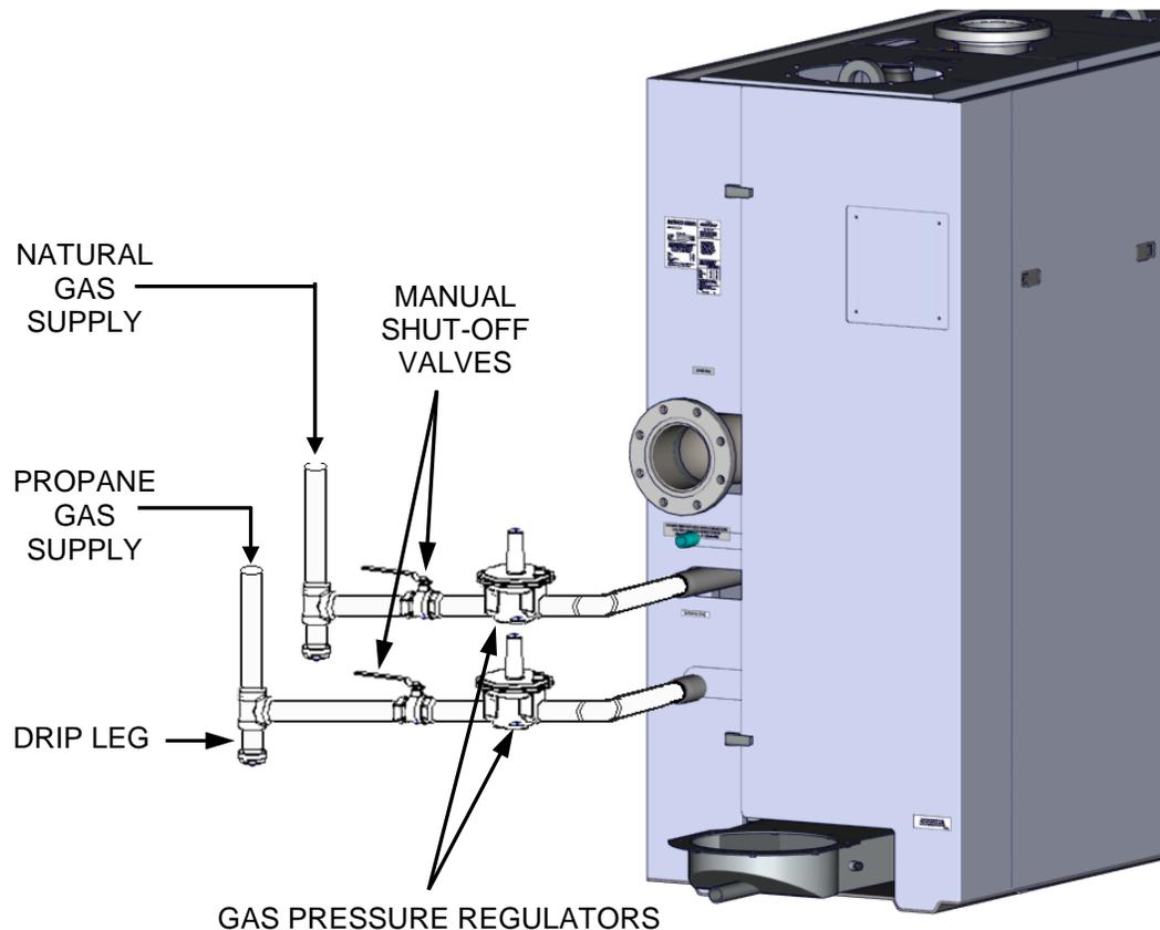
**Figure 2-8. Manual Gas Shut-Off Valve Location**
