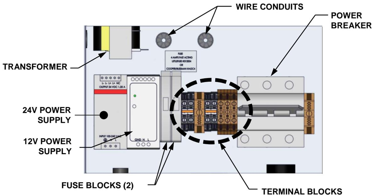
**Figure 2-10. Power Box Internal Components (Cover Removed)**
