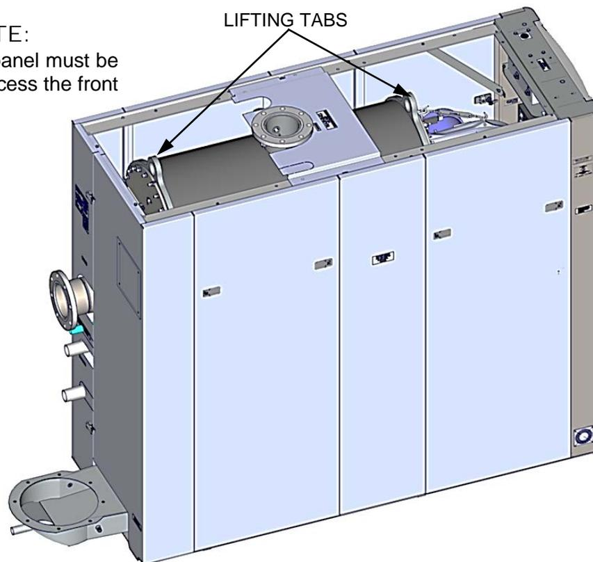
TOP VIEW WITH TWO TOP PANELS REMOVED
