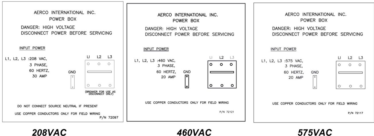
**Figure 2-11: Power Box Cover Labels, 208VAC (Left), 460VAC (Center), 575VAC**
