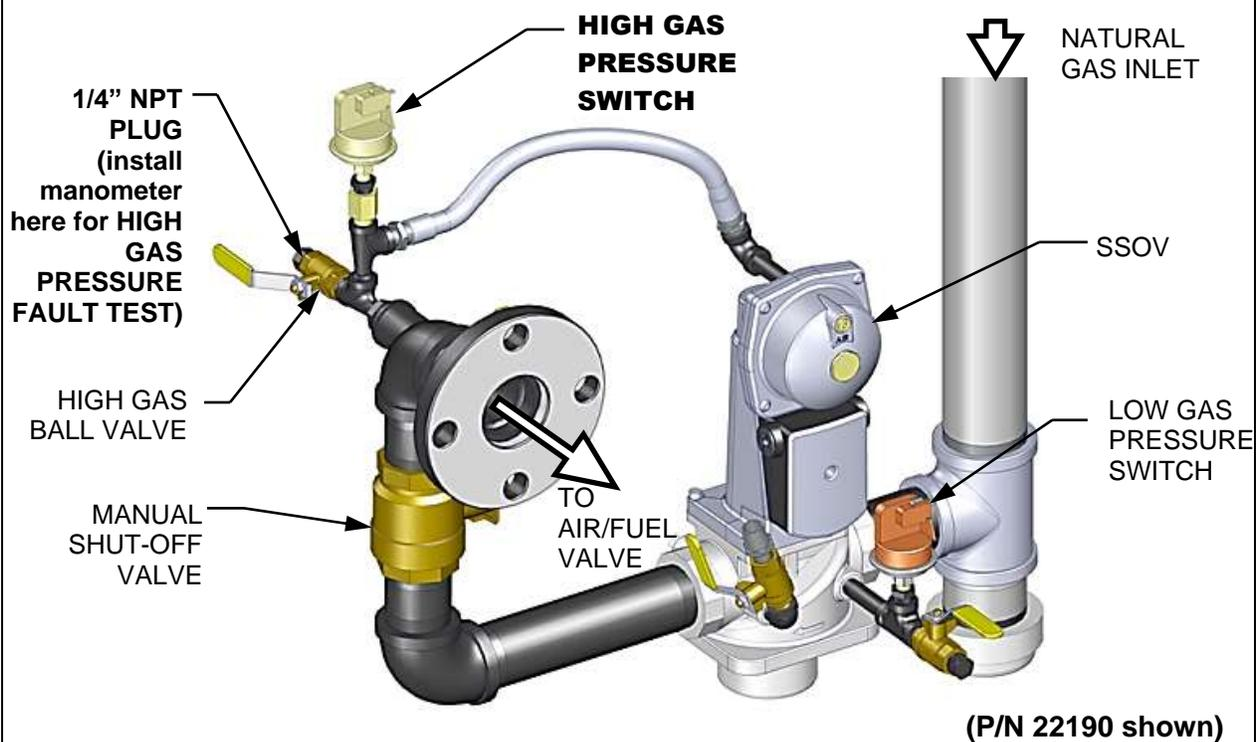
*Figure 5-3c: BMK 2500: HIGH Gas Pressure Fault Test*
