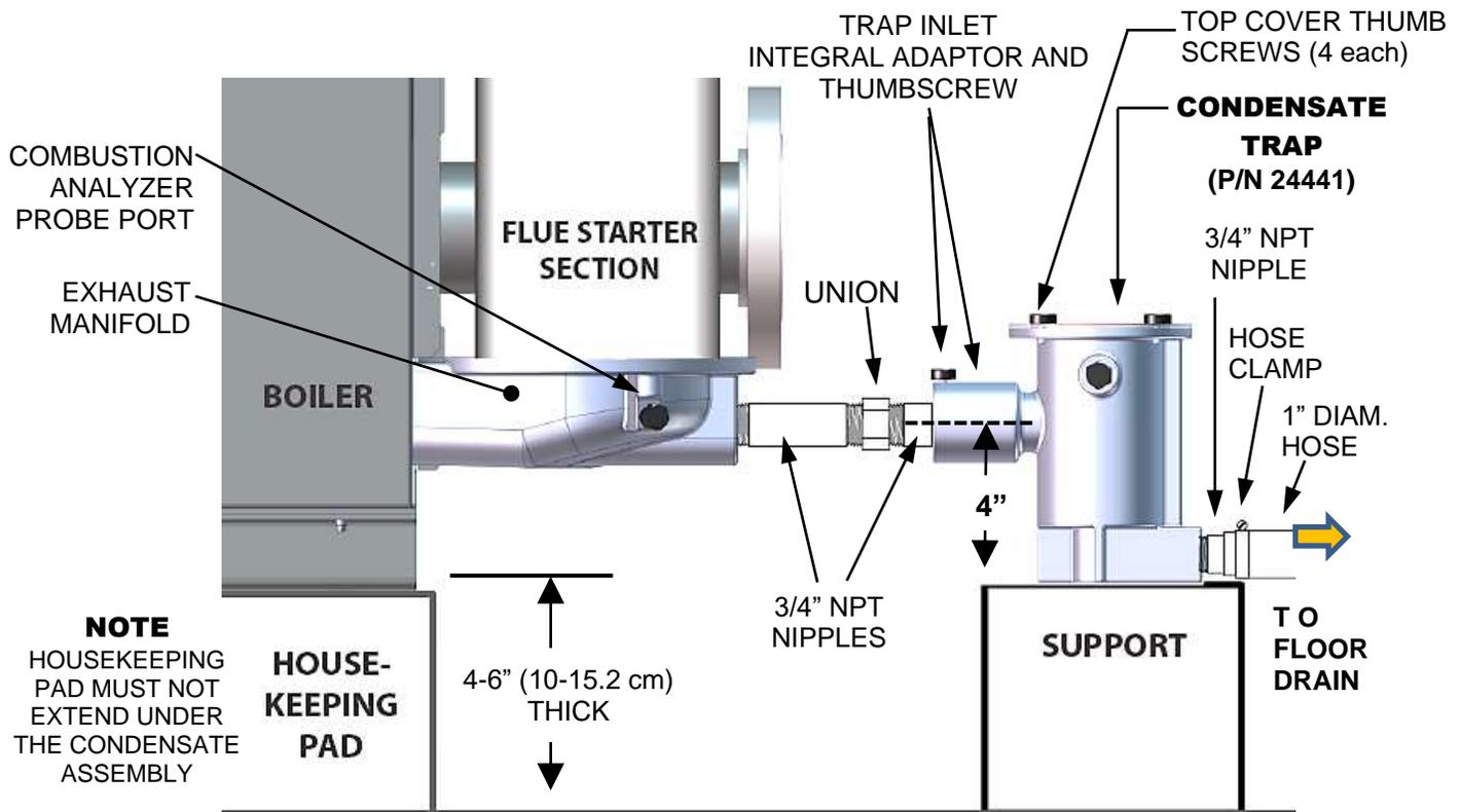
Figure 2-6a: BMK 750/1000 Sample Condensate Trap Installation
