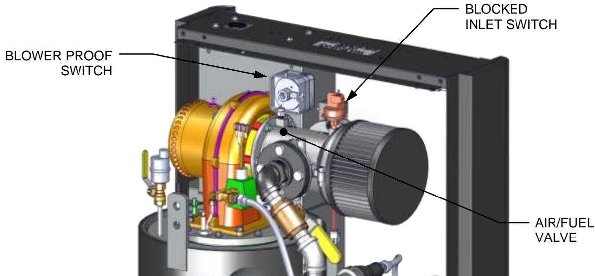
**Figure 5-6b: Bare Boiler – Partial View – BMK 750/13000 Shown**
