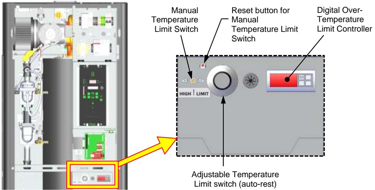
*Figure 5-5b: Temperature Limit Switch Location – BMK 750-1000*
