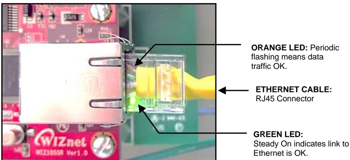
*Figure 7-2: Ethernet Link and Data Traffic LEDs*
