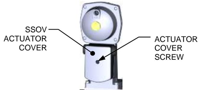
**Figure 5-8: SSOV Actuator Cover Location**
