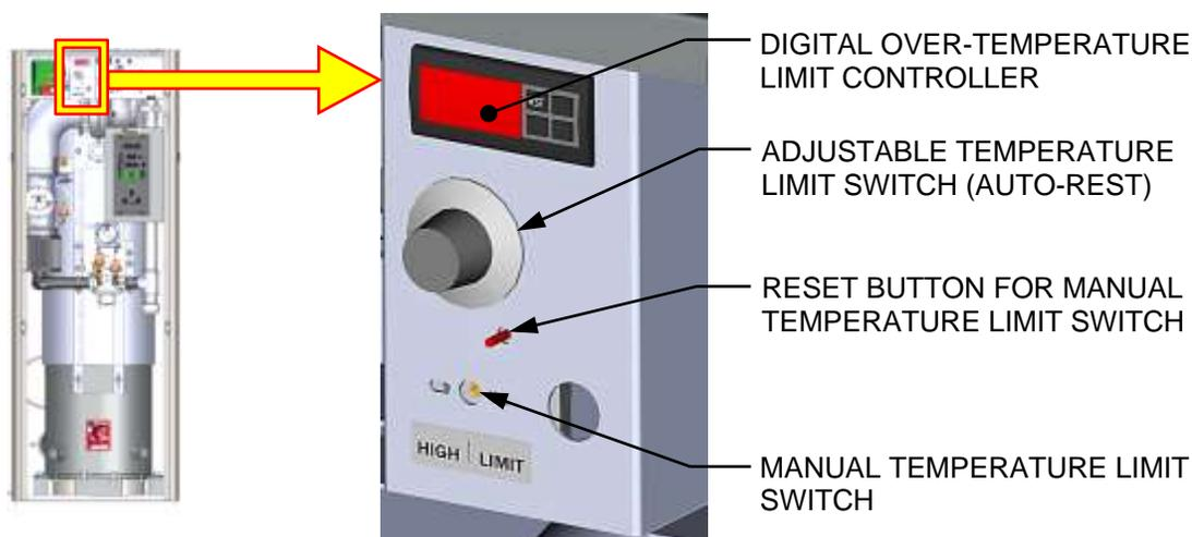
**Figure 4-6b: BMK 1500 – 3000 Over-Temperature Limit Switch Location**
