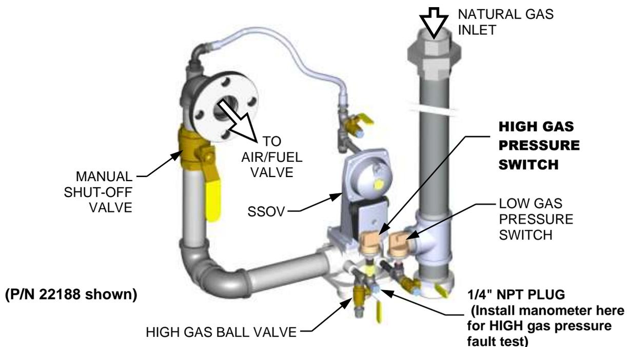
**Figure 5-3b: BMK 1500/2000: HIGH Gas Pressure Fault Test**
