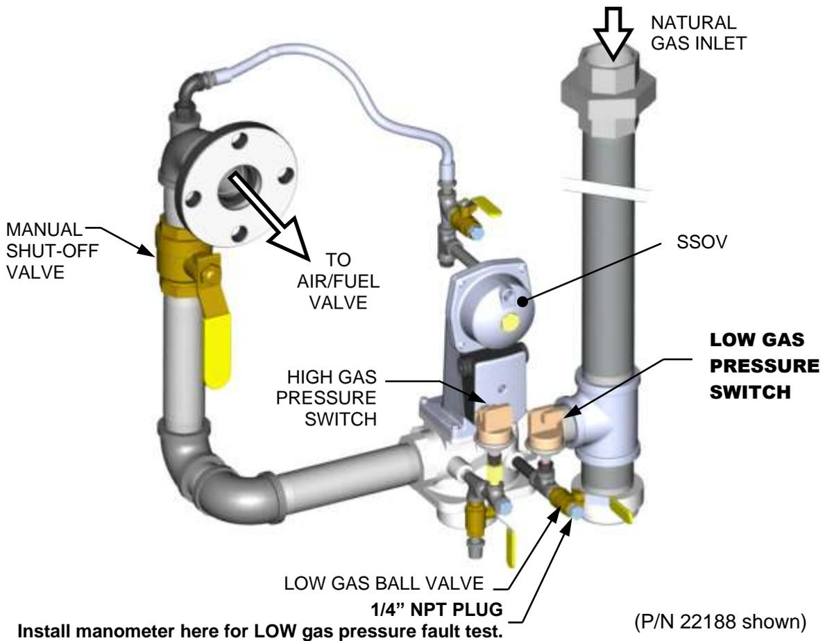
**Figure 5-1b: BMK 1500/2000 LOW Gas Pressure Test Components**
