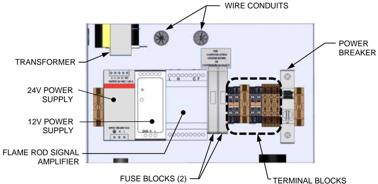
**Figure 2-10b: BMK 1500/2000 Power Box Internal Components**
