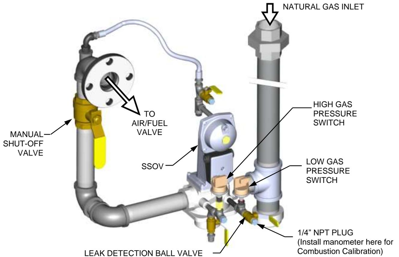
**Figure 4-1b: BMK 1500 & 2000 1/4 Inch Gas Plug Location (P/N 22188 shown)**
