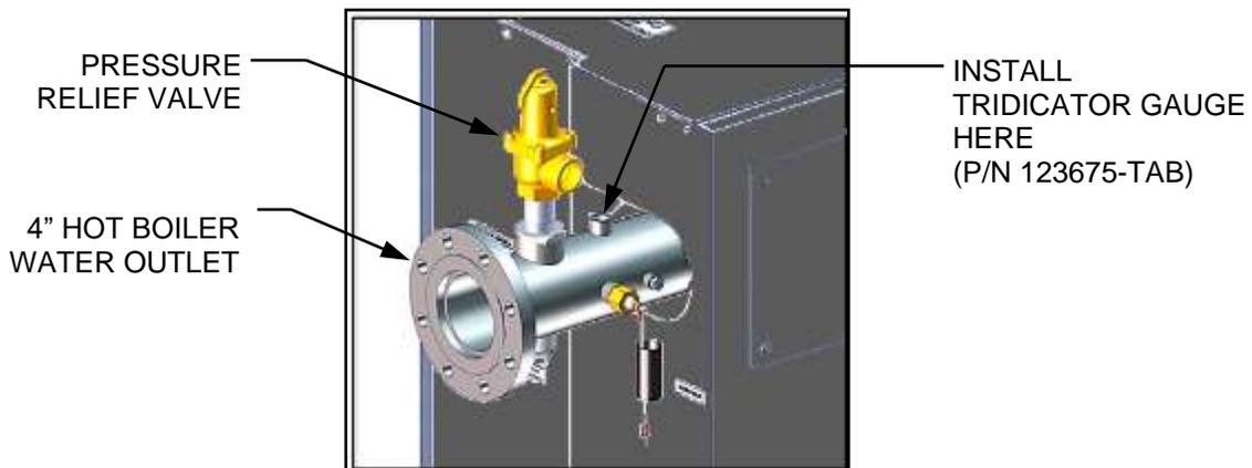
**Figure 2-5b: BMK 1500/2000/2500/3000 P&T Relief Valve Location**
