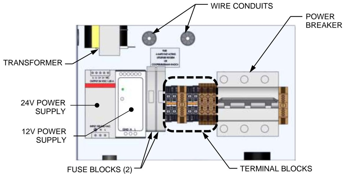
**Figure 2-10c: BMK 2500/3000 Power Box Internal Components**
