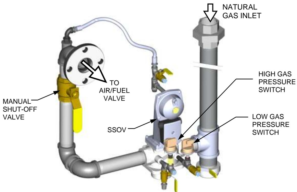
**Figure 3-1b: BMK 1500 & 2000 SSOV Location (P/N 22188 shown)**
