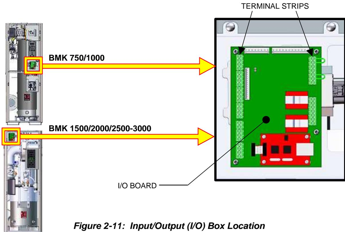
**Figure 2-11: Input/Output (I/O) Box Location**
