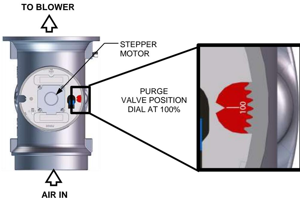
*Figure 3-2b: BMK 1500 – 3000 Air/Fuel Valve In Purge Position*
