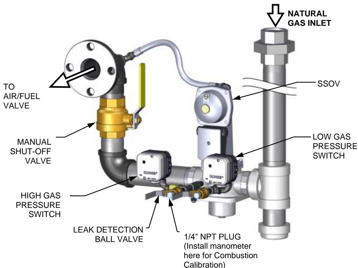
**Figure 4-1d: BMK 3000 1/4 Inch Gas Plug Location (P/N 22171 shown)**
