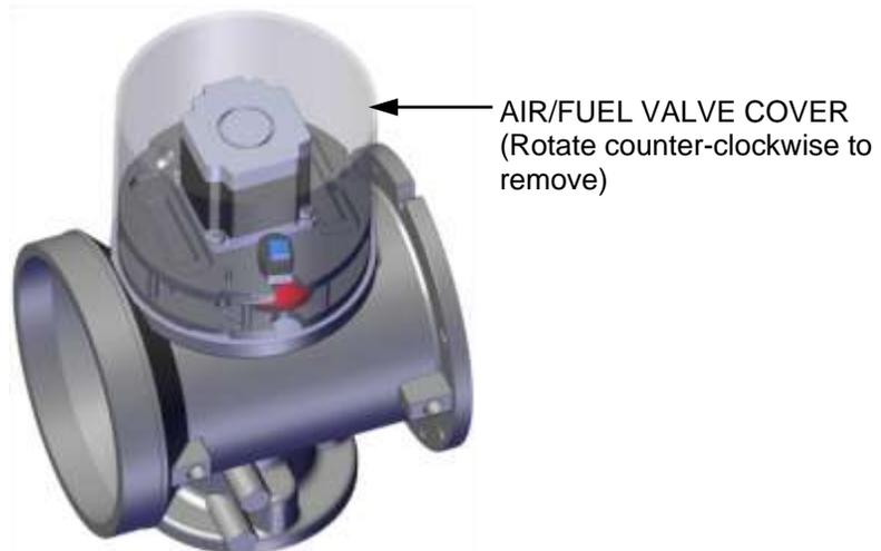
**Figure 5-9b: Air/Fuel Valve Cover Location – BMK 750/1000**
