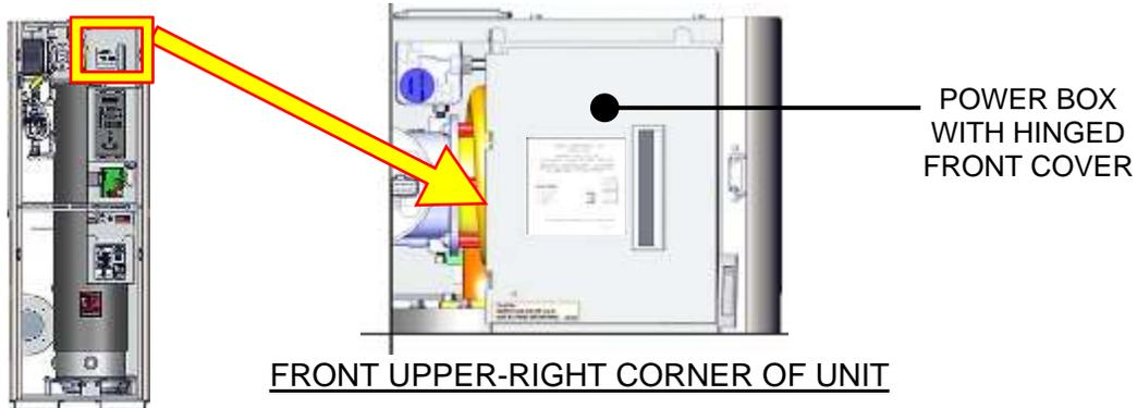
**Figure 2-9a: BMK 750/1000 Power Box with Closed Cover**
