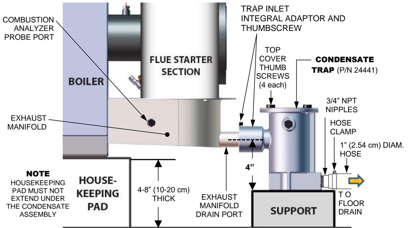
Figure 2-6b: BMK 1500 – 3000 Sample Condensate Trap Installation
