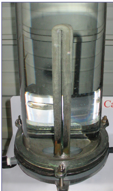
Untreated Scale build-up in untreated water
