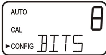
This is the first of three menus to setup the RS-485 parameters. These menus will only appear if the RS-485 mode is selected. Selections are 7 or 8 bits. The factory selection is 8 bits. Make a selection using the ▲ and ▼ buttons then press the ↵ button.
