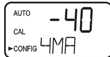
If the 4-20 mA setting is turned ON (7.2 Setting the 4-20 mA Output), the following two menus will appear. The first menu outputs a constant 4 mA while allowing for a small amount of adjustment. The adjustment can be made using the ▲ and ▼ buttons. This adjustment will allow the operator to make the AccUView LED agree with a PLC or SCADA system. The adjustment limits are ± 200 counts or about ± 0.2 mA.
