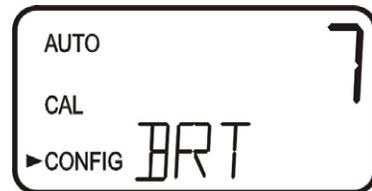
The LCD backlight brightness may need to be adjusted. This is of particular interest if multiple instruments are located in the same area and it is desired for the entire group to have the same appearance. Ten levels are available. The factory brightness is 8.
