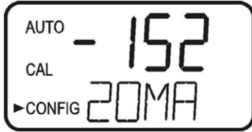
This menu operates similar to the previous menu. This menu outputs a constant 20 mA while allowing for a small amount of adjustment. The adjustment can be made using the ▲ and ▼ buttons. The adjustment limits are  $\pm 1000$  counts or about  $\pm 1$  mA.
