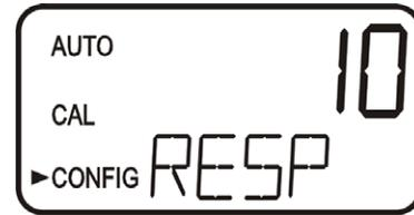
The speed of response for both displayed and output values can be adjusted in this menu. The factory setting is 3 however, 10 response speeds are available. Select the desired speed of response using the **▲** and **▼** buttons. Press the **↵** button to accept it.
