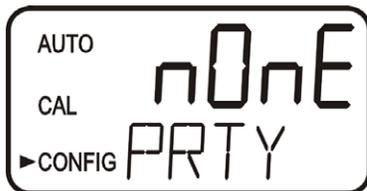
In the Parity menu selections are no parity (nOnE), odd parity (Odd) or even parity (E). The default selection is no parity. Make a selection using the ▲ and ▼ buttons then press the ↵ button. The factory setting is no parity.
