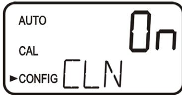
This allows for a selection menu to turn **OFF** the ultrasonic cleaning function if desired. The default mode is **On**. Make a selection using the ▲ and ▼ buttons then press the ↵ button.
