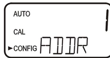
The last selection is the address. This Address is important where multiple instruments are wired on a single string. Each instrument **MUST** have a unique Address.
