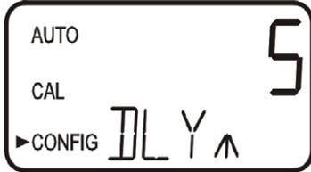
The current selected number of seconds will be shown. Select the desired number of seconds for the "delay on" time for this alarm using the **▲** and **▼** buttons. Once the desired delay time has been set, press the **↵** button to accept it.
