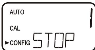
For stop bits the choices are 1 or 2 stop bits. The default selection is 1 stop bit. Make a selection using the ▲ and ▼ buttons then press the ↵ button. The factory setting is 1 stop bit.
