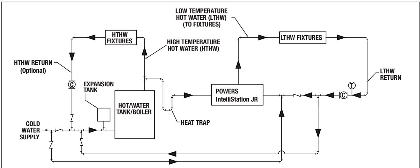
Ⓢ Select flow rate as necessary to ensure Powers IntelliStation JR is operating at an ASSE 1017 minimum certified flowrate. See Literature.
